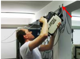
Test person localizing a Co-60 source (red arrow) hidden in a cable rack with the HPGe detector "Micro Detective"
