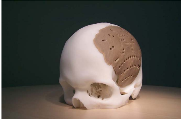
Patient specific implants using SLS process
