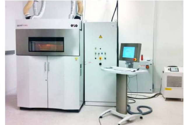
OPM process based on EOS P800 SLS machine technology
