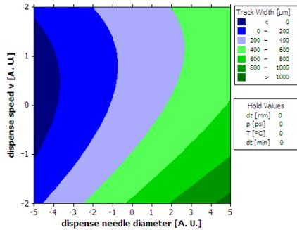
**Figure 5:** Simplified contour plot, given in coded values, for DoE-related screening of deposition parameters: in this case wet film track width in dependency of dispense needle diameter and dispense speed ( $v$ ).
