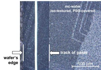
**Figure 6:** Examples for a dispensed track of paste (width:  $\sim 500 \mu\text{m}$ ).
