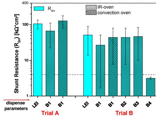
**Fig. 10:** Average values for shunt resistances for different batches of paste isolation vs. reference obtained from validation trials. Dashed line shows minimal value for  $R_{sh}$  required order without significantly diminishing performance of solar cells [3].
