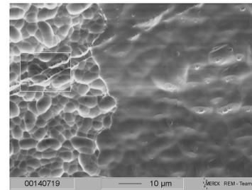
**Figure 7:** SEM-image of the transition area on a mc-wafer after being etched (right) by a deposited track of paste. The paste was deposited on the rear side directly next to the edge of the wafer.
