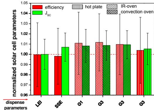
**Figure 8:** Comparison of average conversion efficiencies as well as of  $J_{sc}$  for paste-isolated vs. reference batches processed at ISE.
