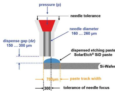
Figure 2: Schemed set-up of lab dispensing system.
