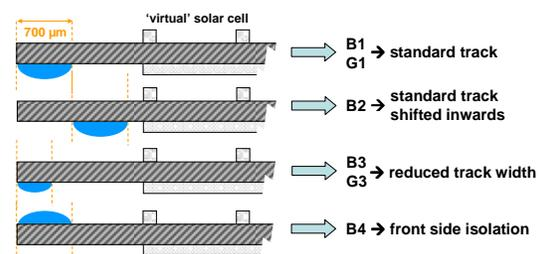
Fig. 4: Sketch demonstrating various dispense parameters and paste depositions.
