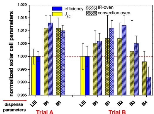
**Figure 9:** Average values for conversion efficiencies as well as for  $J_{sc}$  for different batches of paste isolation vs. reference obtained from validation trials.
