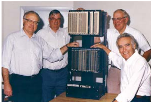
1968: Bedford Associates, Modicon 084 (MODular Digital CONTroller)
