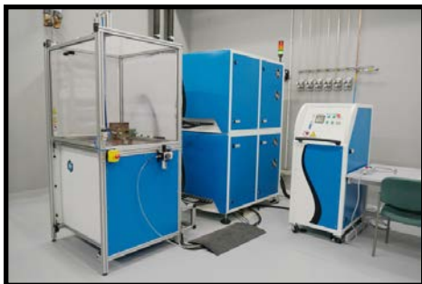
Bmax MPW50/25: single turn coil, integrated \varnothing 42 mm field shaper
