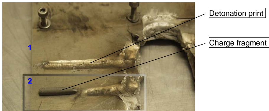
Fig. 7 Witness plate results for full (1) and for interrupted (2) detonation
