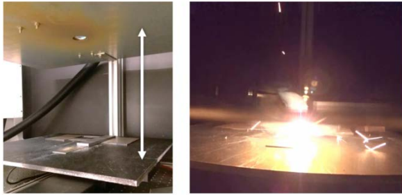
Figure 4: Determination of acceptable plume heights by a setup with an adjustable cover sheet. Left: setup. Right: welding process.
