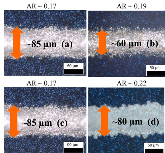
**Figure 3:** Microscope pictures of a screen printed contact finger (3a, 3d) processed within process A (see Figure 1) and a screen printed contact finger (process B in Figure 1) after seed layer printing (3c) as well as of a screen printed contact finger after light induced plating (3d) is shown. Mean values of the finger width and the aspect ratio are given.
