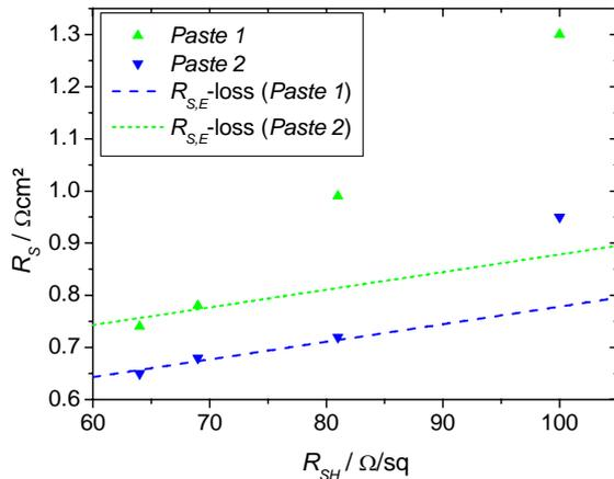
**Figure 4:** Series resistance  $R_{\text{S}}$  of the solar cell plotted against the emitter sheet resistance  $R_{\text{SH}}$  for two different front side silver pastes. The dashed lines show the linear influence of series resistance losses of the emitter  $R_{\text{S,E}}$  calculated with the formula presented in (1).
