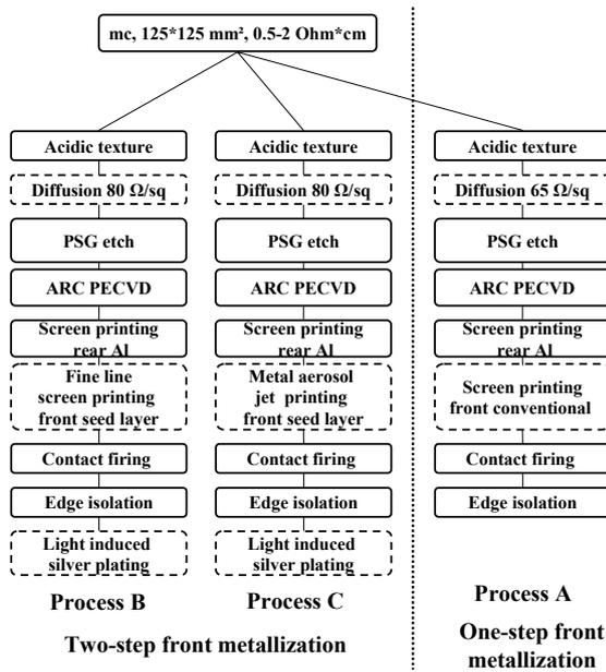
**Figure 1:** Process flow of conventional mc-Si solar cells with a one- (process A) or two-step front metallization process (process B and C). All process steps which are varied, for example the front printing process, are marked (dashed boxes).
