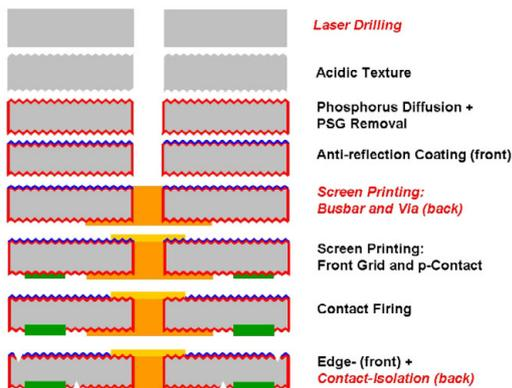
**Figure 2:** Process flow for mc-Si MWT solar cells. All additional or modified process steps compared with the conventional solar cell process are *in italics*.
