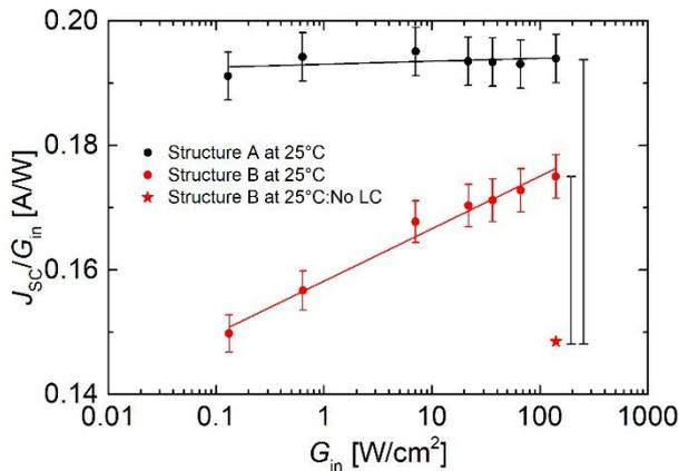
Fig. 1. Measured spectral response  $SR=J_{sc}/G_{in}$  at  $\lambda_0=809 \text{ nm}$  and  $25 \text{ }^\circ\text{C}$  for structure A and B. The red star represents the estimated value in absence of luminescence coupling.
