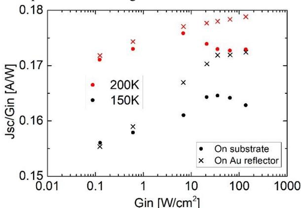
Fig. 2. Measured spectral response of multi-junction cells with structure A, at  $\lambda_0=809 \text{ nm}$  and at temperatures of  $150 \text{ K}$  and  $200 \text{ K}$ , *i.e.* below the design temperature of  $25 \text{ }^\circ\text{C}$ . Measurements are carried out for cells on substrate and cells with Au reflector.
