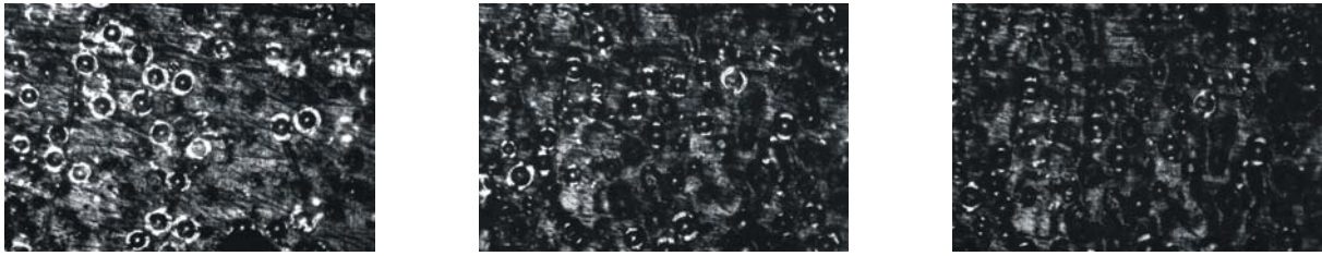
Figure 1: Light microscopy – Matrix-filler detachment
