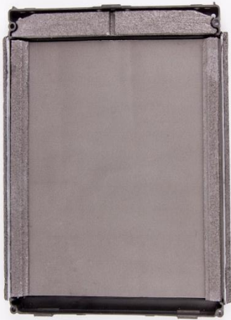
Fig. 3 Frame including PGS foil and PCM inlays
