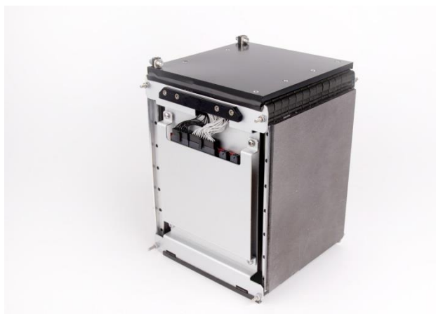
Fig. 2 Battery module prototype
