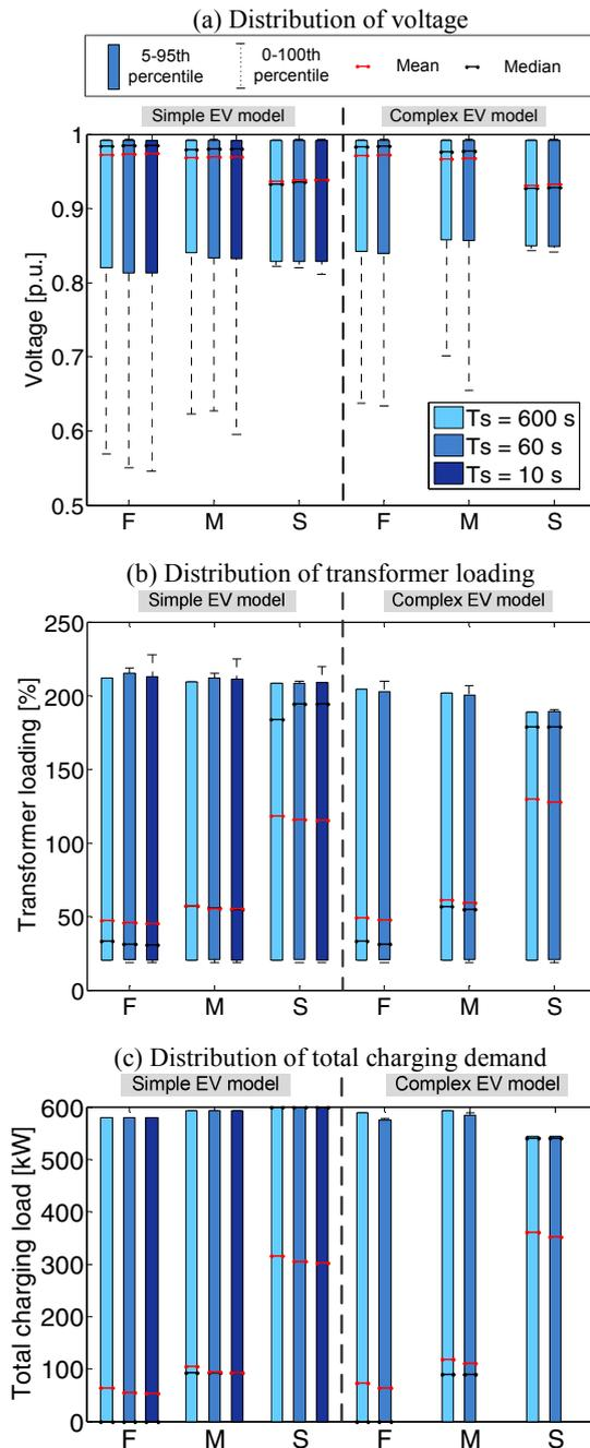
Fig. 9: Statistical summary of simulation results on the worst case scenario. F, M, and S: Fast, mixed and slow charging mode, resp.
