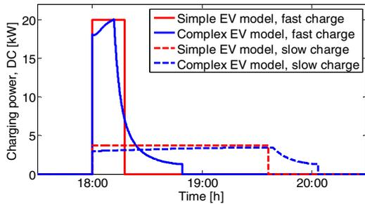
Fig. 4: Typical charging curves of different EV models and charging modes.
