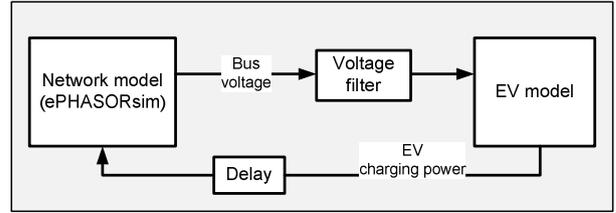
Fig. 7: Schematic diagram of simulation model
