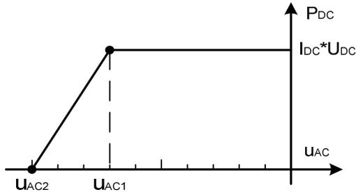
Fig. 3: Characteristics of the AC voltage controller in the complex EV model.
