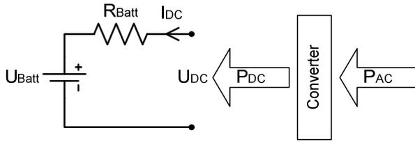
Fig. 2: Schematic diagram of the complex EV model.
