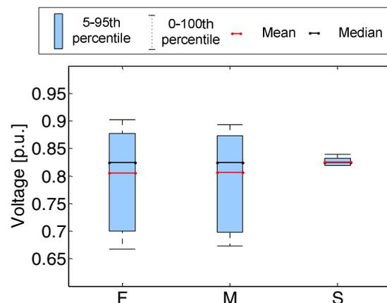
Fig. 5: Distribution of grid voltage minima by variation of EV charging positions with maximum EV penetration.
