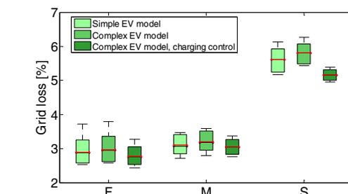
Fig. 10: Results of sensitivity analysis on charging pattern F, M and S: Fast, mixed and slow charging mode, respectively.
