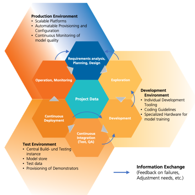
Figure 1: The MLOps cycle [Beck et al. 2020].
