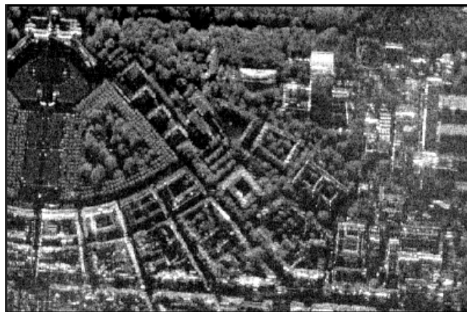
Fig. 9. SAR image (X-Band, HH-Pol., approx. 1m ground resolution)
