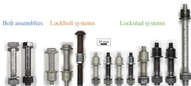
Figure 2 Representation of the investigated fasteners
