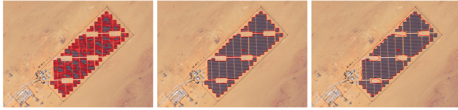
Figure 4.2: Comparison of segmentation results at different resolutions for the Reggane PV system. From left to right: 20, 80, and 320 cm. The red overlay shows the results from segmentation.
