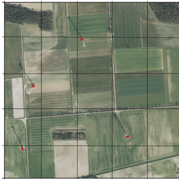
Figure 6.2: The method of the static cutting of the training images is shown. The black lines represent the cutting edges, the red dots the coordinates of the wind turbines.
