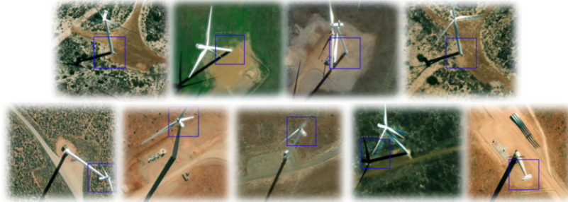
Figure 6.7: True positive examples from the application using the Bing images are presented as follows. The upper row displays instances featuring clearly visible and accurately identified wind turbines, where the centroid of the regression boxes serves as the base of the tower. The bottom row, shows correctly identified wind turbines, with less accurate regressive delineation in the images.
