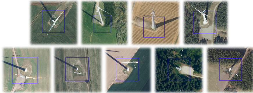
Figure 6.6: True positive examples from the application using the DOPs images are presented as follows. The upper row displays instances featuring clearly visible and accurately identified wind turbines, where the centroid of the regression boxes serves as the base of the tower. The bottom row, shows correctly detected wind turbines, with less accurate regressive identification on the images.
