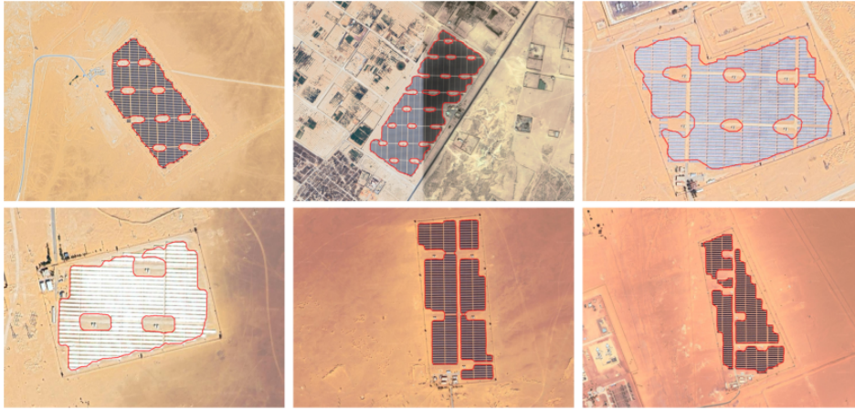
Figure 4.4: Satellite imagery with segmentation results for the PV systems in the Piat region. Red outlines indicate the predicted PV areas. From left to right and top to bottom: Timimoune, Adrar, Z Kounta, Kabertene, Aoulef, and In Salah.
