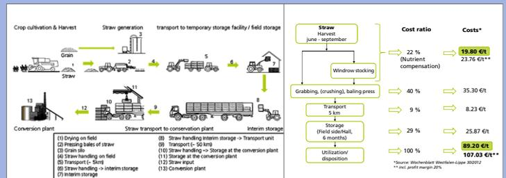
Fig. 1: logistic chain for straw recovery
