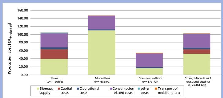
Fig. 4 : share of cost components for different biomass feedstock
