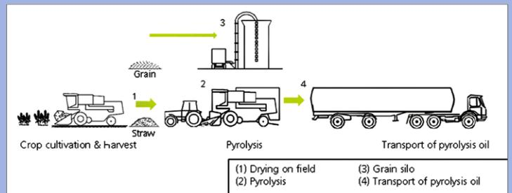
Fig. 3: logistic chain for mobile pyrolysis
