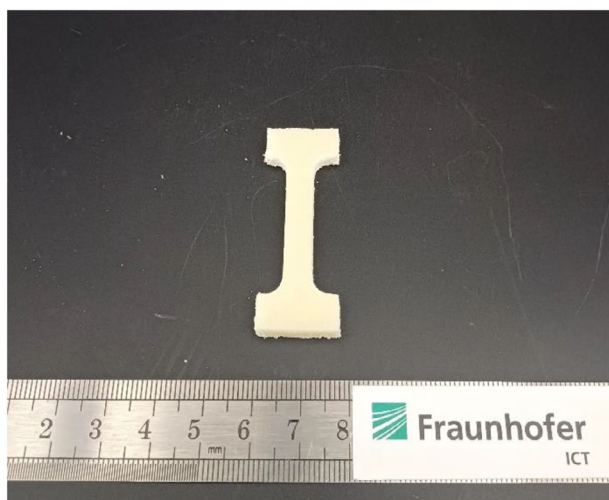
FIGURE 2 | Dog bone specimen of the NFPEG3N3 plasticized formulation.
