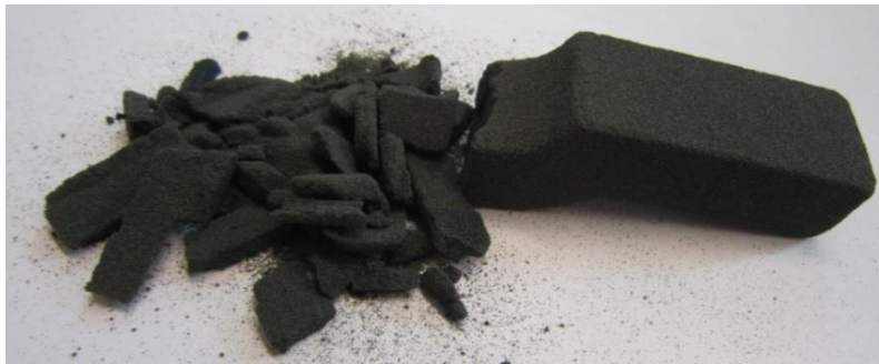
Figure 7: Broken specimen from furan resin-bonded sand (not infiltrated)
