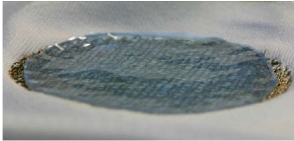
Figure 9: embroidered circular electrode with solid gel pad for better skin contact.
