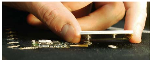
Figure 4: the flat battery can be removed for washing and charging.
