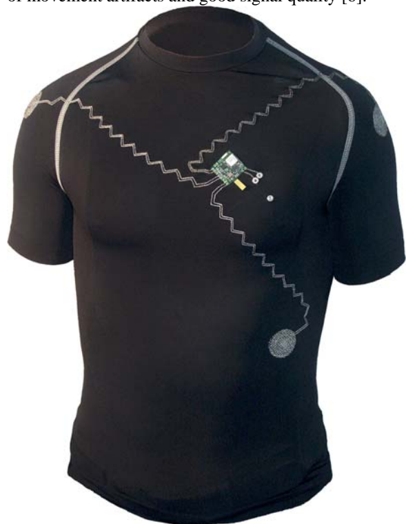
Figure 5: the shirt with electronics, snap fasteners for the battery and embroidered electrodes and conductors.
