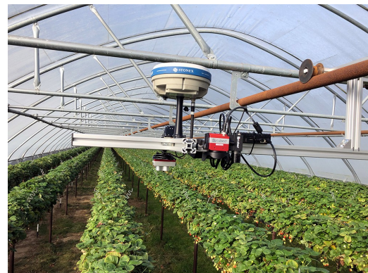
Figure 1: Strawberry plants cultivated under a poly-tunnel and imaged using a hyperspectral camera mounted on a moving rail mechanism
