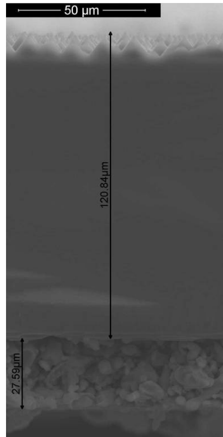
Figure 8. A picture of a complete section of the cell has been taken with a SEM, from this image it can be realized that the features like texture and metal layers begin to play a significant role on the total geometry of the cell at the thickness used in this work.
