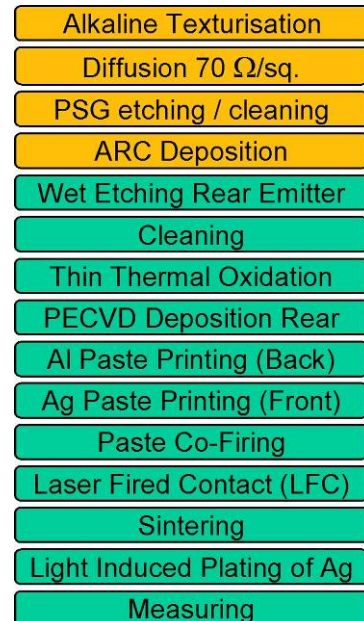
Figure 2. The process flow is depicted here. The processes performed at Deutsche Cell GmbH are highlighted in orange while in green the ones performed at Fraunhofer ISE are presented.
