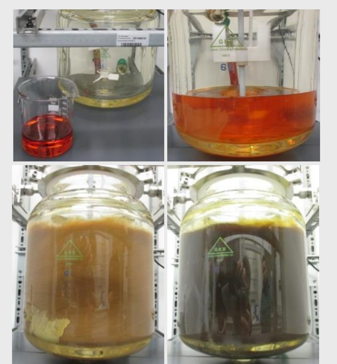
Fig 5. Synthesis of TAAILs (left) and extraction process (right); (TU Dresden)
