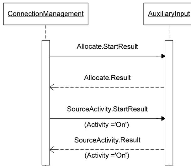
Figure 1 Example of a specified sequence for a successful startup of an Auxiliary Input [6]
