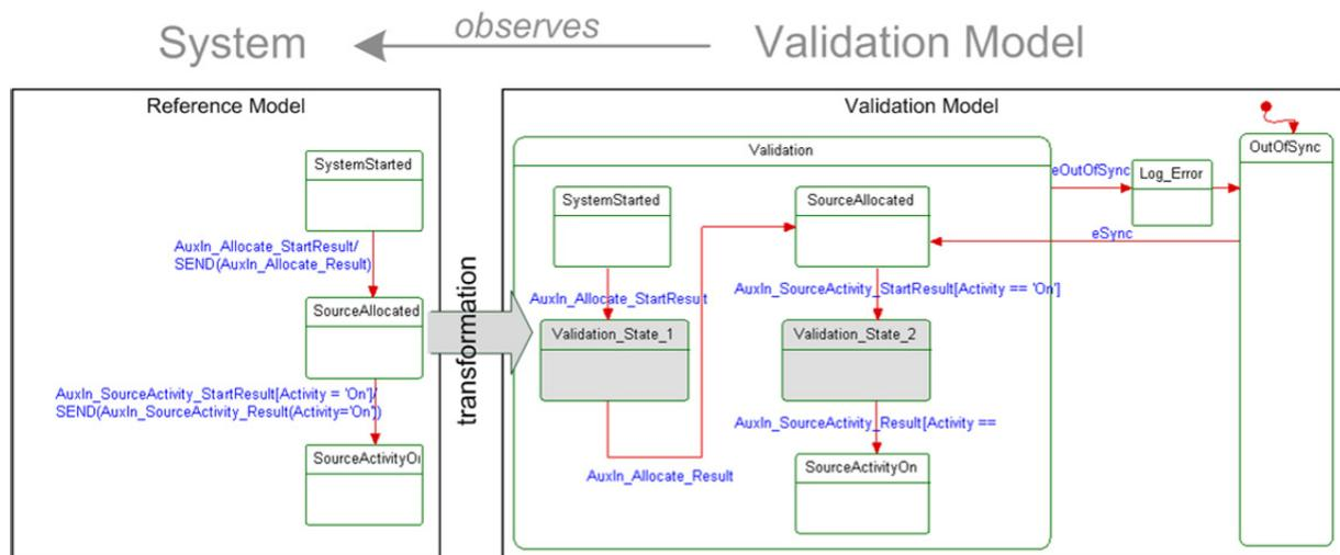
Figure 3 Validation model of the AuxiliaryInput Function Block [5]
