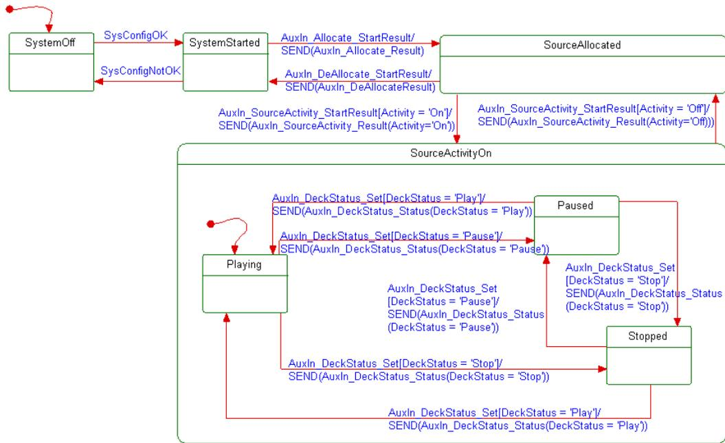
Figure 2 Example of the specification model for the Auxiliary Input Function Block [5]
