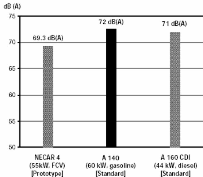
Figure 8: External noise emission of NECAR 4 and standard Mercedes-Benz A-Class vehicles at the standardized “accelerated passage” test (measured in IDIADA for the “accelerated passage” test, defined by the European regulation 70/157/EWG) [8]
