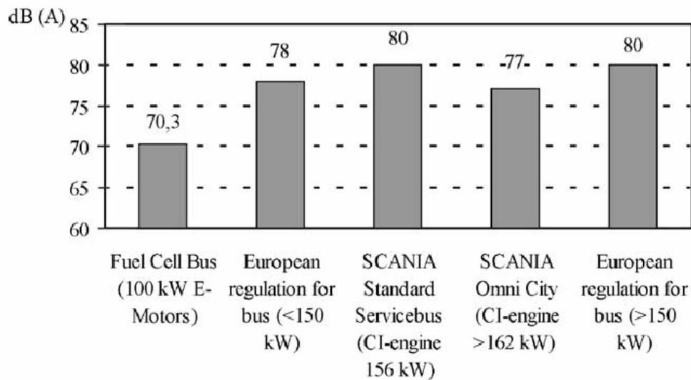
Figure 10: Results from noise measurements, defined by the European regulation 70/157/EEC [12]
