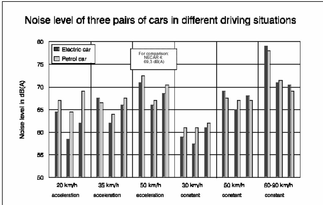
Figure 9: Noise level of three pairs of vehicles in different driving situations [9].
