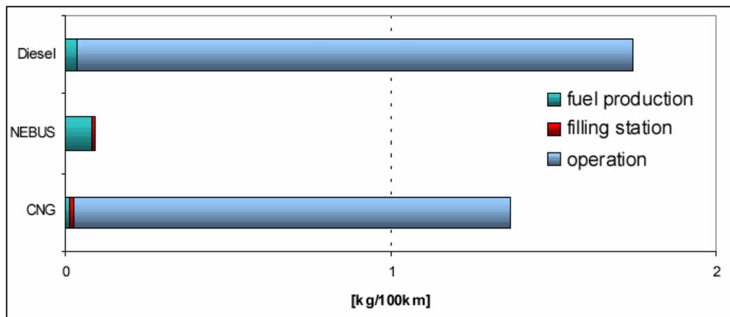
Figure 13: NO<sub>x</sub> emissions in urban drive cycle
