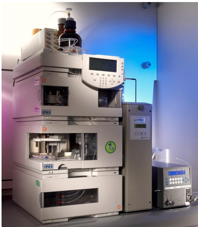
Figure 19: Agilent Technologies 1100 Series coupled with PSS ETA-2010 detector used for Gel Permeation Chromatography
