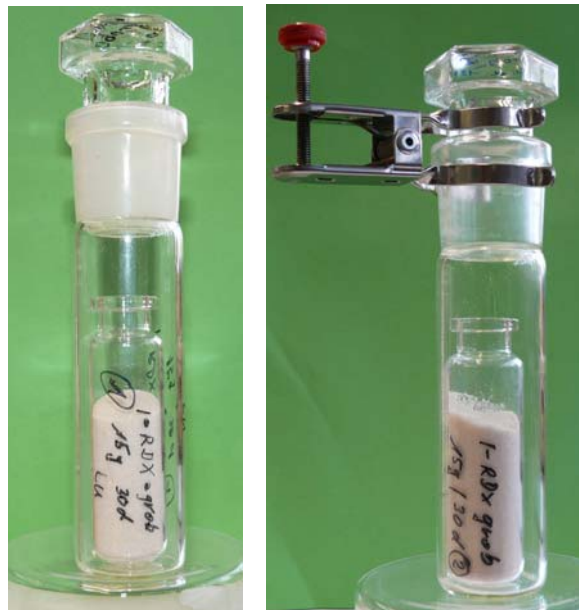
Fig. 5.1: Ageing of RDX samples in small vials inserted in the ageing vials. Left: ageing in air, not sealed stoppers, regularly opening of the vials to let fresh air in. Right: Ageing under argon with sealed stoppers and clamped to avoid lifting of stoppers by internal over pressure.
