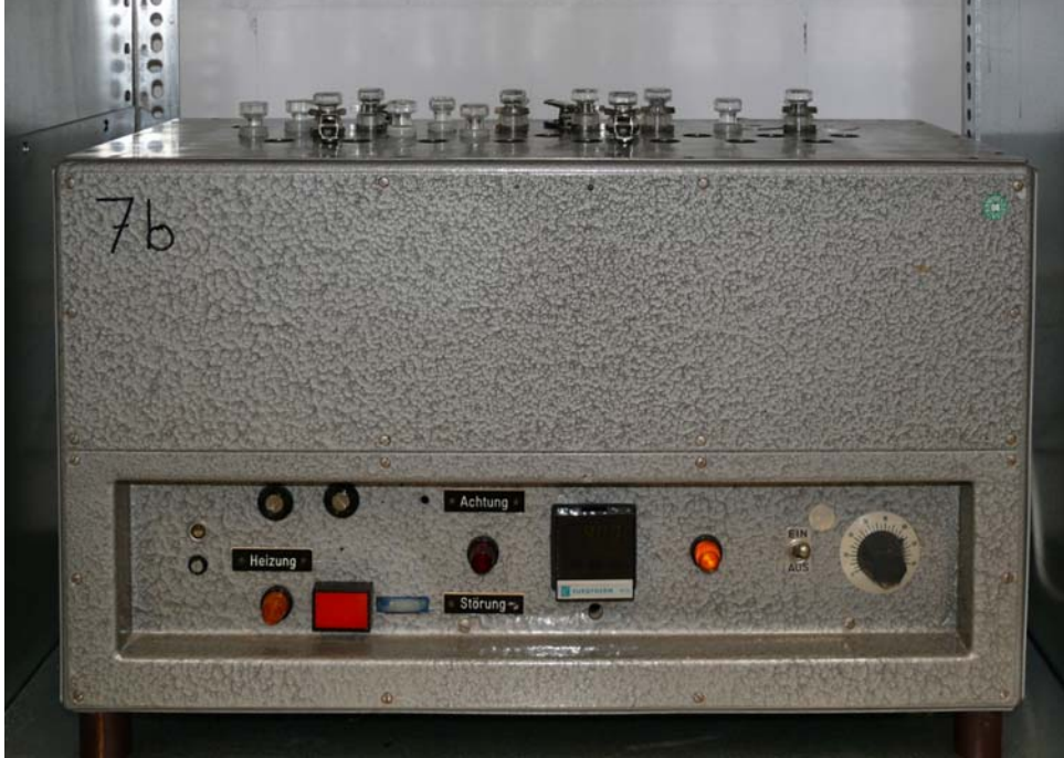
Fig. 5.2: Example of a PID temperature controlled aluminium block oven for ageing of samples in vials.
