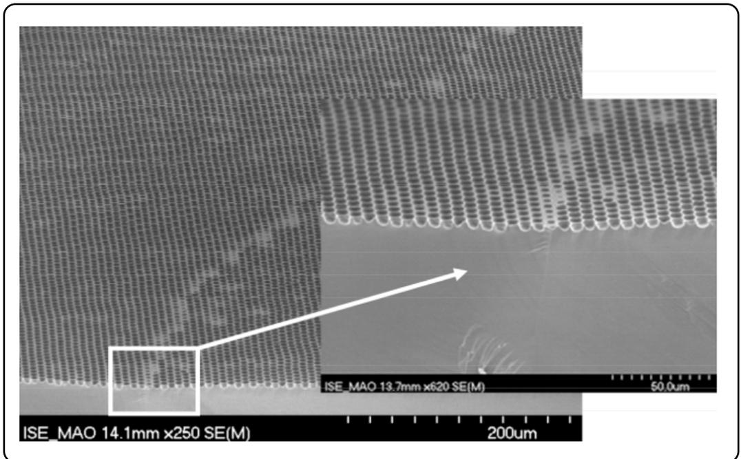
**Figure 2** – Honeycomb textured mc-Si wafer after NIL and plasma etching. Shown is a magnification of a grain boundary.
