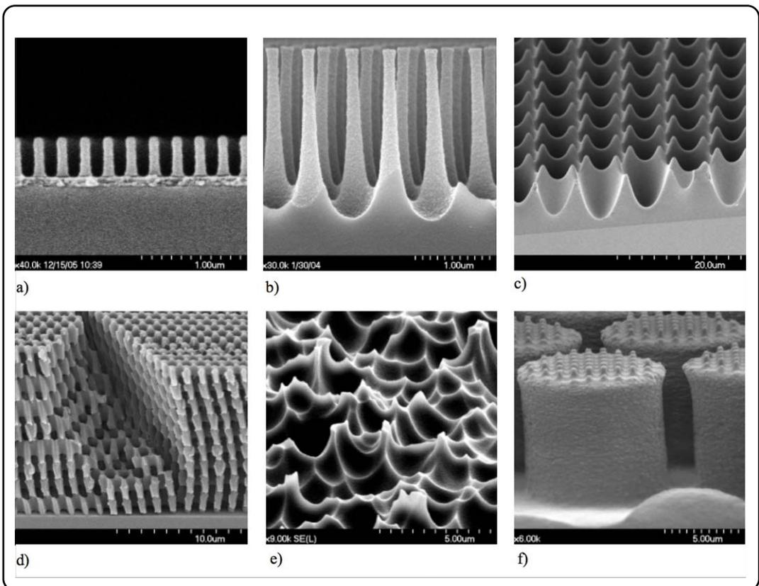
**Figure 1** – Structures originated by interference lithography: a) linear grating (two wave interference); b) crossed grating with high aspect ratio (combination of two exposures, each with two waves); c) honeycomb structures (three wave interference); d) photonic crystal (four wave interference); e) surface-relief diffuser (multi-wave interference); f) combination structure for enhanced adhesion, inspired by the feet of geckos (three-wave interference plus double two-wave exposure)
