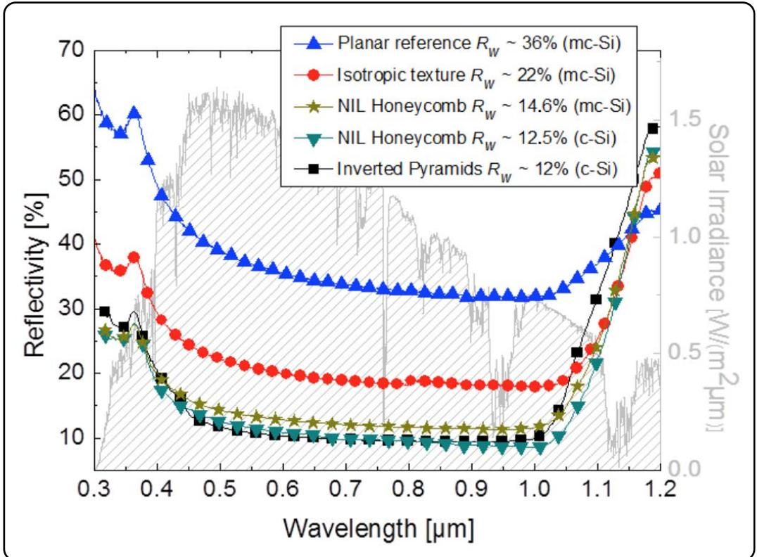
**Figure 2** – Reflection measurements of differently textured substrates. The honeycomb texture realized by the presented process chain was characterized on c-Si as well as on mc-Si.[9]
