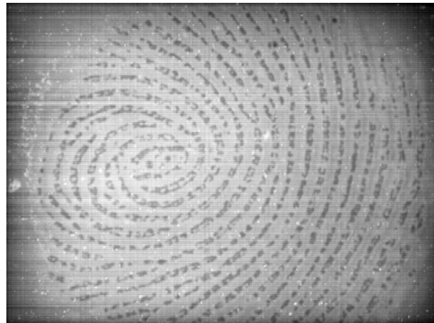
Figure 11. Bidirectional microdisplay in fingerprint application, captured fingerprint sample.
