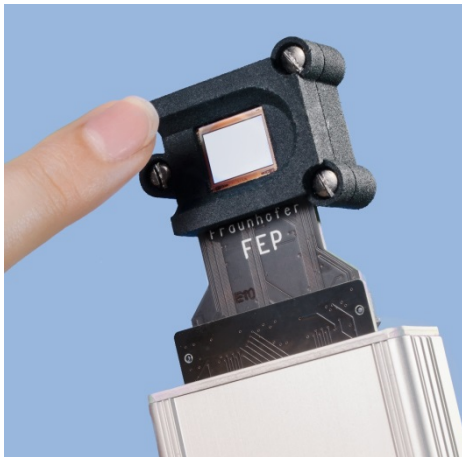
Figure 11. Bidirectional microdisplay in fingerprint application, captured fingerprint sample.
