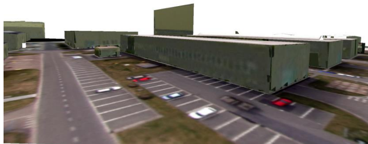
Figure 8: 3D-terrain model of area with texture from orthophoto for pixel on horizontal areas and from slant view video for pixel of vertical areas (walls).
