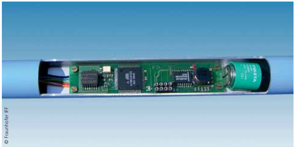
After the javelin has been thrown, data from the integrated chip is transmitted to a laptop.
