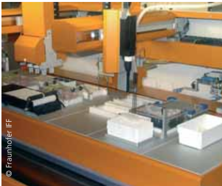
TELOMICS™ ex vivo robotics from KeyNeurotek AG, the first fully automatic system for tissue screening.
