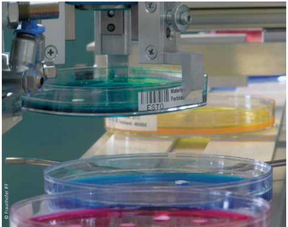
MIROB, the robot for AnagnosTec GmbH for automatic sample preparation of microorganisms.
