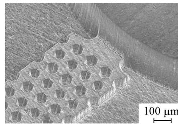
Figure 2: Fluid structure in SiC
