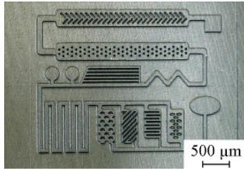
Figure 3: Fluid forming tool in SiC
