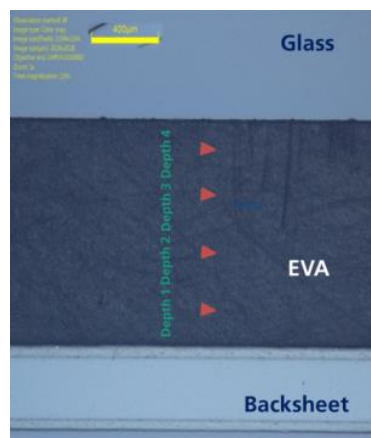
Figure 7: Microscopic images of the cross-section of the glass/EVA/BS laminate. Red triangles indicate the measurement points (depth) lateral from 1 (closest to backsheet) to 4 (closest to glass).
