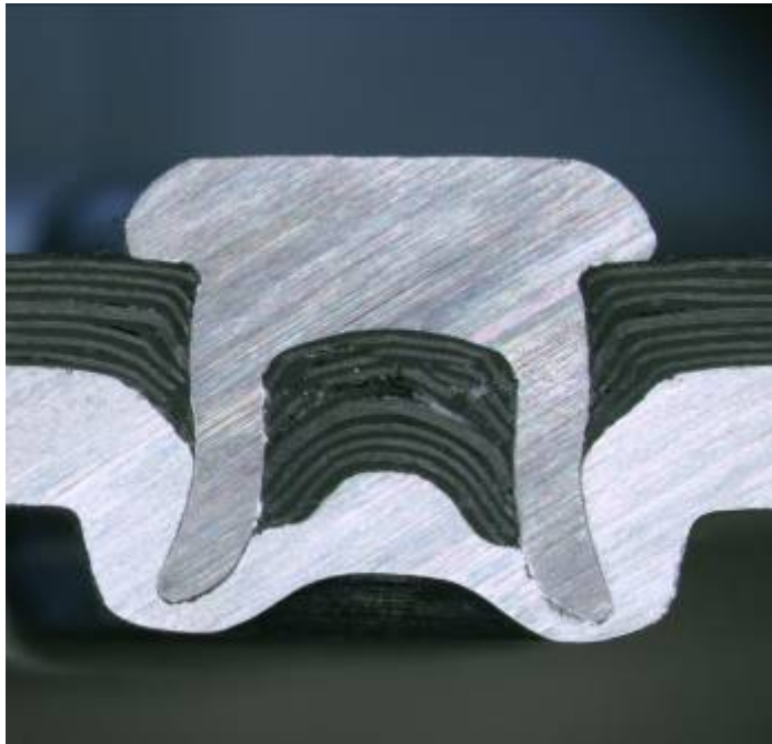
CFK T700SC/RIM935-[0/90]4S (2,1mm) in AlMgSi0,5 T6 (2,0mm)
