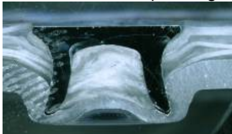
Semi-tubular self piercing rivet joint
