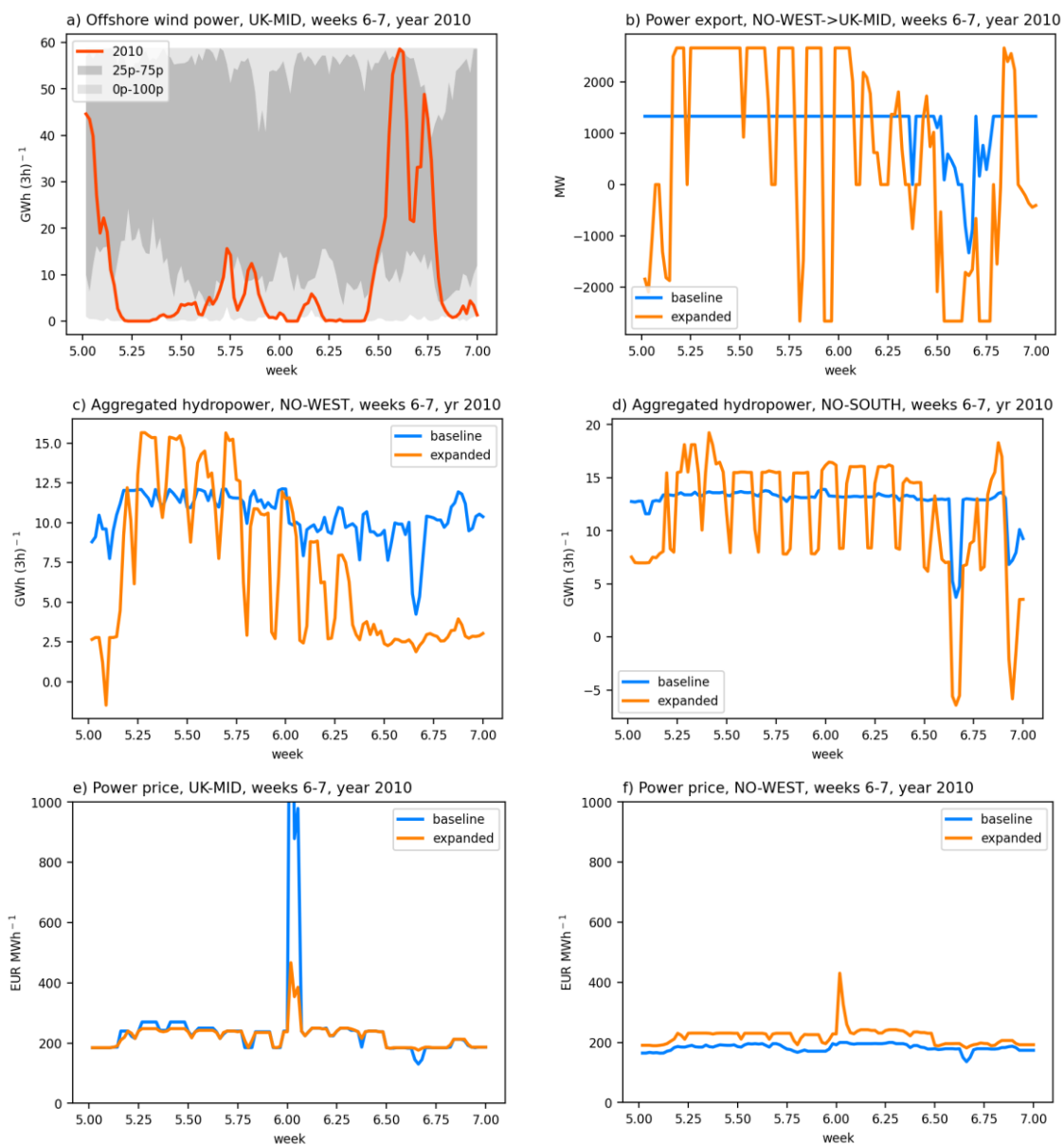
Figure 4. Example FanSi results illustrating a periodical energy shortage based on simulations for weeks 6-7 in 2010. Panel a shows offshore wind power for UK-MID (these data are model inputs and thus the same in 'baseline' and 'expanded'). "0P-100P" denotes 0-100 and "25P-75P" 25-75 percentiles range across 30 simulated weather years. Panels b-f compare 'baseline' and 'expanded' scenario results for power export from NO-WEST to UK-MID (negative values mean import to NO-WEST), aggregated hydropower in NO-WEST, and power price in UK-MID and NO-WEST, respectively. See Figure 1 for definitions of areas.
