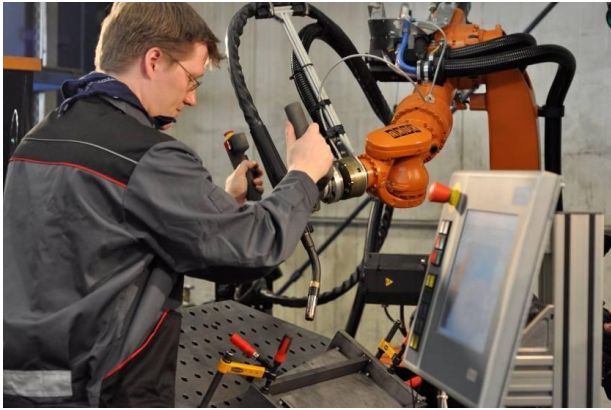
Figure 1 Inteach system for intuitive programming of welding applications
