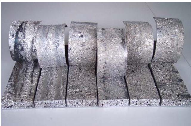
Fig. 5: Selected peeling samples after the peeling experiment (from left to right: A1, B1, C1, D1, E1, H1)
