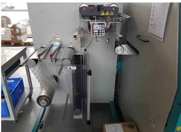
Figure 1: Unrolling the antenna inlay foil, which enters through the slit on the right hand side into the assembly chamber. The foil is highly charged at the assembly point, if no countermeasures are made.
