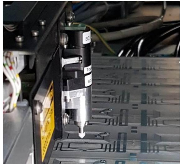
Figure 9: Placement unit with non-dissipative nozzle; no ionizer in place, although it should be at this process step.
