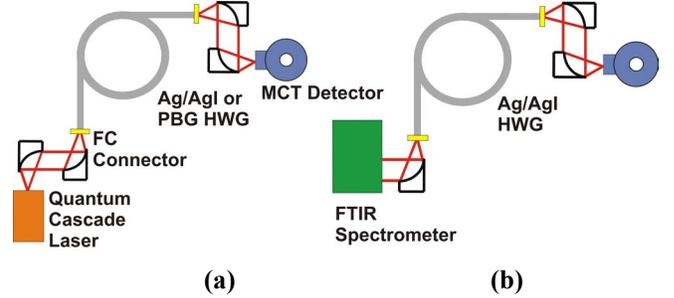
Figure 2. Evaluation of hollow waveguides using (a) a quantum cascade laser, and (b) a FT-IR spectrometer.
