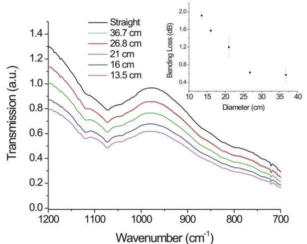
Figure 5. FT-IR-based transmission measurements of Ag/AgI coiled hollow waveguides. The inset shows the bending losses inside conventional hollow waveguides vs. the coil diameter.
