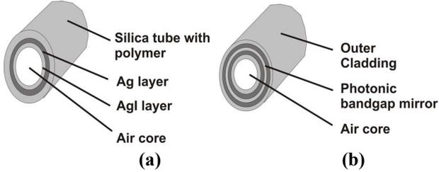
Figure 1. Schematic structure of (a) conventional hollow waveguide, and (b) photonic bandgap hollow waveguide.
