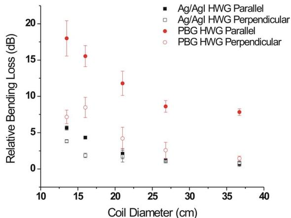
Figure 4. Experimentally determined total loss in conventional and photonic bandgap waveguides using a quantum cascade laser. The nomenclatures “parallel” and “perpendicular” indicate relative relationship between the polarization direction of the laser radiation and the plane of bending. The plane of bending is defined as the plane where the coiled waveguide exists.
