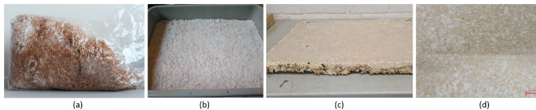
Figure 1. Mycelium cultivation and growth. (a) Inoculation of substrate using mycelium in growth bag; (b) growth of the material in a polypropylene (PP) growth box; (c) living mycelium after approximately 14 days of growth. (d) Zoom of the mature mycelium and the growth structure.
