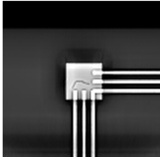
Figure 7. Circuit board phantom, frontal view, magnified, left SART, right AP-SART using registered a priori volume.
