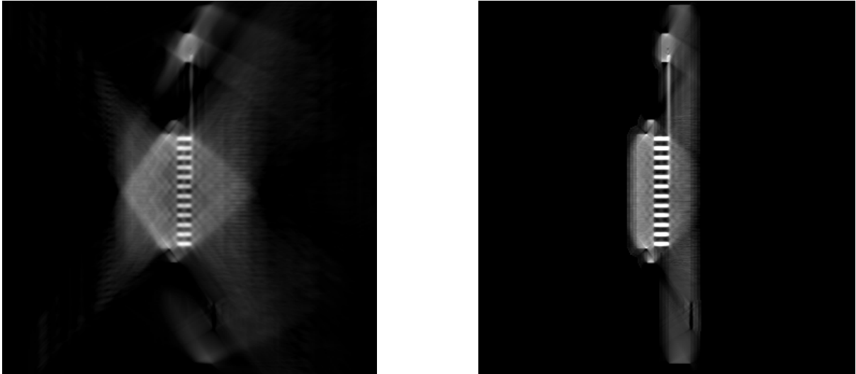
Figure 8. Circuit board phantom, lateral view, left SART, right AP-SART using registered a priori volume.
