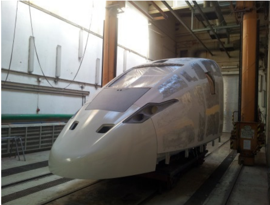
Figure 4: Demonstrator before coating with paint, with add-on parts made of GRP; like front, wiper case, shell for front and side lights
