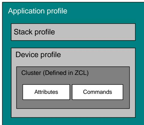
**Figure 4** Structure of ZigBee's profiles
