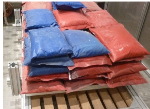
Figure 5: Test setup with sandbags at -40 °C
