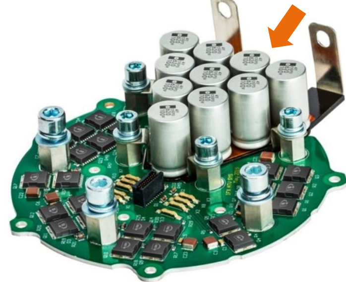
RONG Rui, „AN-Power stage of 48V BSG inverter Reference design with TOLL & TOLG MOSFET“, www.infineon.com , 2018
