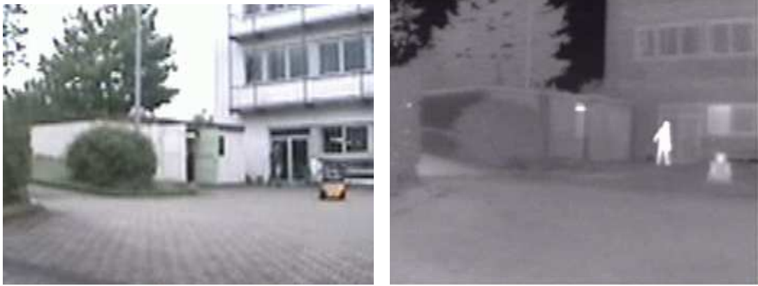
Figure 1. Same scene in VIS (left) and LWIR band (right). The person can be discovered more easily in LWIR than VIS.
