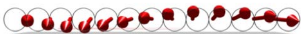
Basic concept of a spin wave. The red arrows are the magnetic moments
