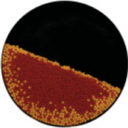
Figure 1. Asymptotic size segregation result in a tumbler mixer. The small particles segregate to the centre. Whereas, the large particles concentrate in the periphery region. Experiment from [10]
