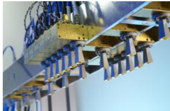
Fig. 1. Sparse line array based 3D terahertz imaging system.
