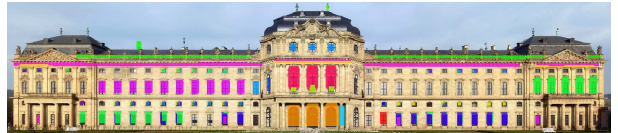
Fig. 7. Facade reconstruction based on automatically generated hypotheses without hierarchical clustering based redundance filtering. The background label class was not visualized, to highlight the foreground background separation.
