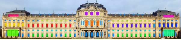
Fig. 8. Facade reconstruction based on automatically generated hypotheses with hierarchical clustering based redundancy filtering. The background label class was not visualized, to highlight the foreground background separation.
