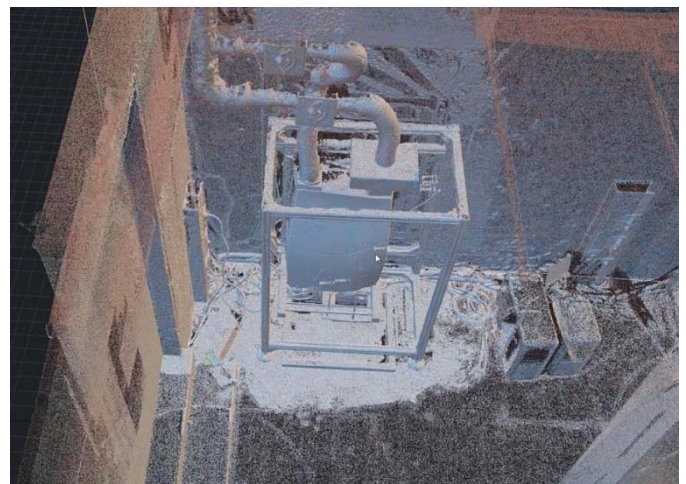
Fig. 7. Integration result of Photogrammetry model (Nikon D810 D2) and point cloud of laserscanner
