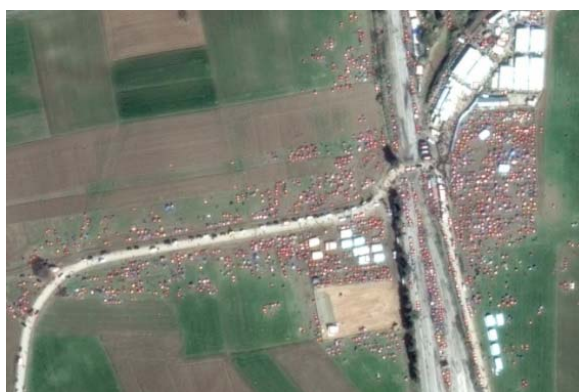
Fig. 3. The output of the Faster R-CNN. The input satellite image of a refugee camp located in Idomeni (Greece) was analyzed. The red bounding boxes mark the dwellings found by the Faster R-CNN. Figure taken from [1].
