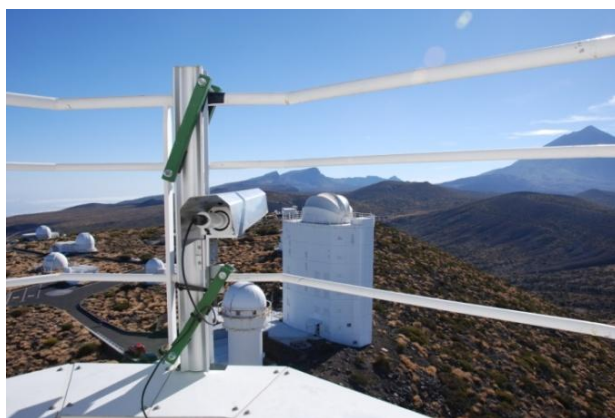
Figure 2. Receiver of laser-scintillometer SLS40 on top of the GREGOR tower, viewing towards the transmitter on the VTT at telescope level 30 m above ground.
